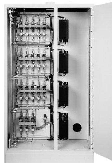
Rear tube-pull source cabinet with vertical gas panels
